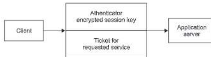
Figure 9.14 Communication between the client and the application server.
